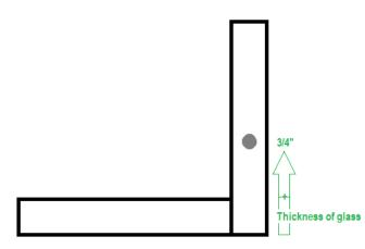
Go in 3/4" + thickness of glass to find hole placement
